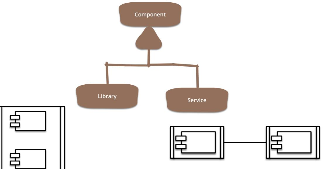
Libraries run within a single process, communicating through language function call mechanisms Services run in separate processes, communicating with networking mechanisms such as HTTP or TCP/IP
